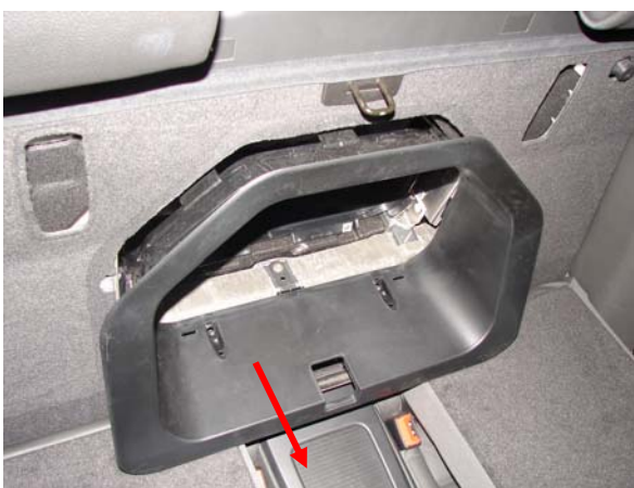
Picture 5: remove the plastic frame
