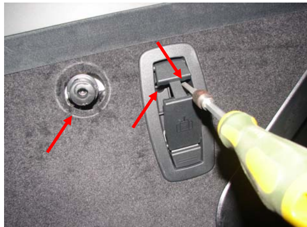
Picture 2: remove plastic rings using a flat screwdriver, loosen 2 torx TX20 screws
