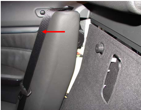
Picture 7: remove side part of the rear seat, it is clipped
