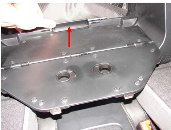
Picture 3: push the lever (red arrow) backwards and remove the separation
