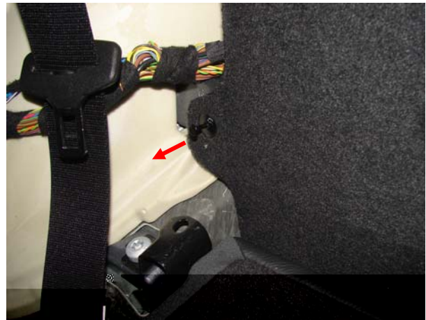
Picture 8: pull out plastic pin to remove plastic rivet
