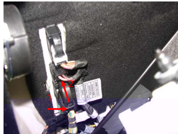
Picture 10: remove connector: pull down latch (arrow 1), then turn strap to the top (arrow 2)
