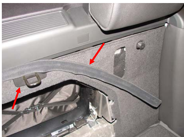
Picture 6: remove the sealing ledge and the plastic cover
