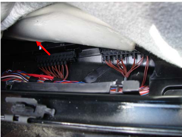
Figure 5: open cable channel, CAN-Distributor
