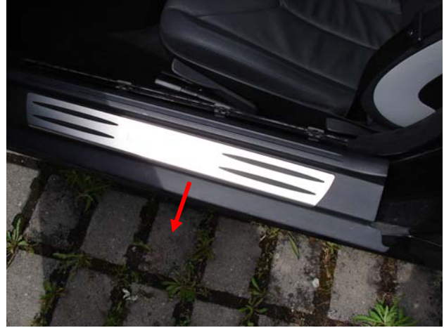
Figure 2: pull sideways to remove cover
