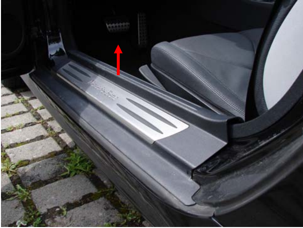
Figure 1: pull up to loosen cover
