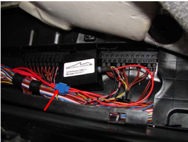
Figure 9: +12V connection of CMR171
