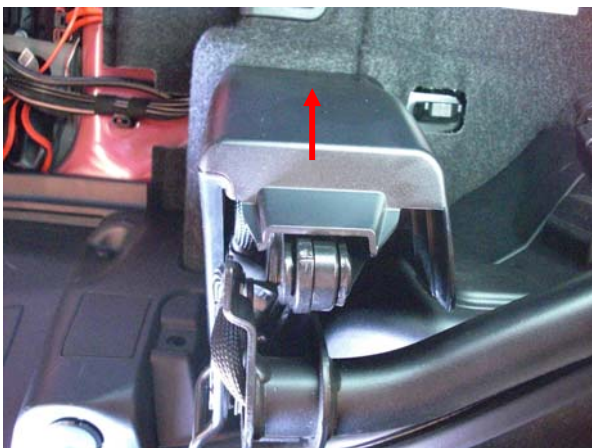
Picture 3: remove cover, pull in the arrow's direction
