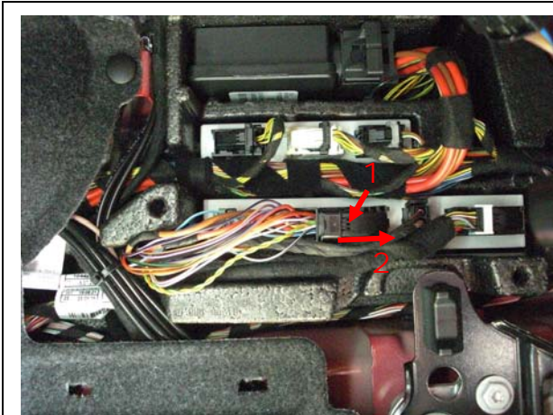
Picture 9: remove connector: pull down latch (1), then turn strap to the right (2).
