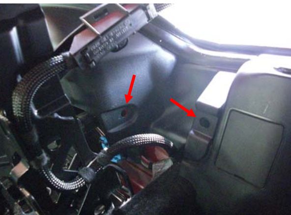
Picture 5: remove two plastic rivets
