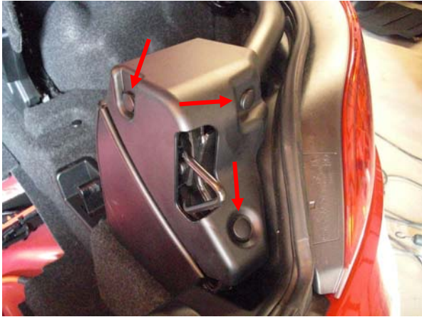
Picture 1: passengers side: remove three plastic rivets
