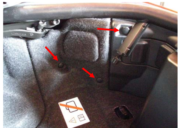
Picture 4: passengers side: remove three plastic rivets
