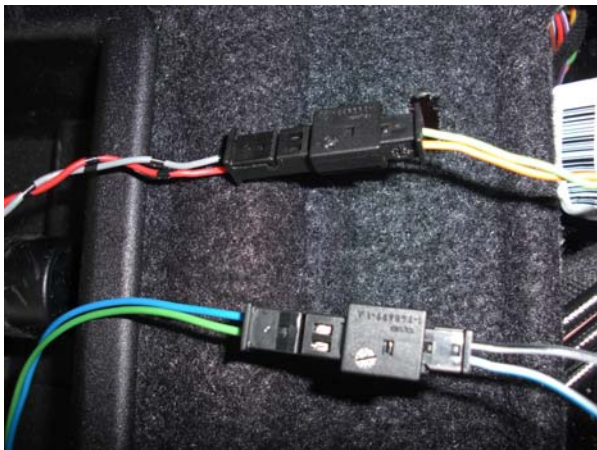
Picture 13: plug the removed wires into the 2-pole connector housings:
