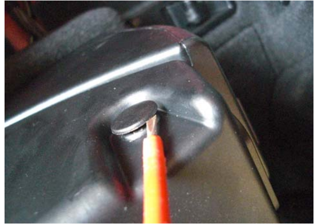
Picture 2: pull out plastic pin to remove plastic rivet
