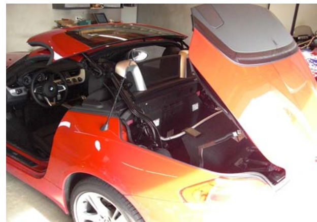
Picture 6: open the roof and stop it in this position, then turn ignition off
