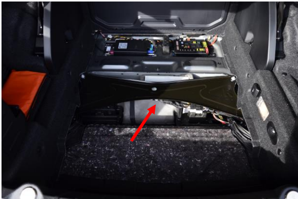
Image 1: Remove the trunk mat, Roof control unit is in the middle under the black cross strut (red arrow)
