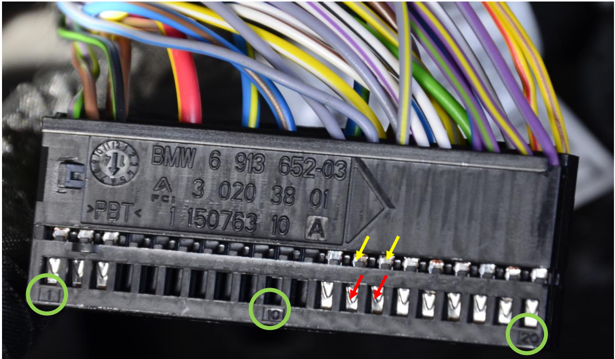
Image 4: Cable gray / blue (gray with blue stripe, pin 13) and gray / yellow (gray with yellow stripe, pin 14) from the plug. On the other side of the connector, the yellow / red (pin 40) and yellow / brown (pin 41) cables must be pulled out of the connector. To do this, press the locking lug down with a screwdriver (red arrow), then pull the cable out a little and press the locking lug down again (2nd lock) (yellow arrow). Now the cable can be pulled completely out of the plug. The pin numbers are printed on the connector (green circles).
