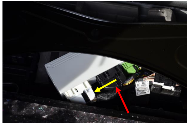
Fig. 2: Loosen the black plug: press the latch (red arrow), then fold the bracket to the left (yellow arrow)
