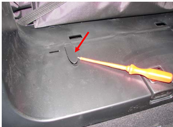
Picture 4: remove covers and then the screws behind it
