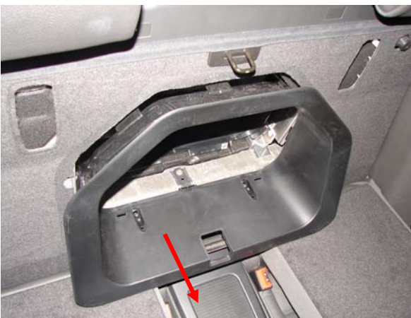
Picture 5: remove the plastic frame
