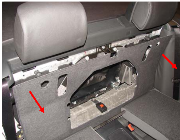
Picture 9: cover is multiple clipped, pull it in the shown direction
