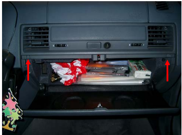
Picture 2: loosen 2 screws
