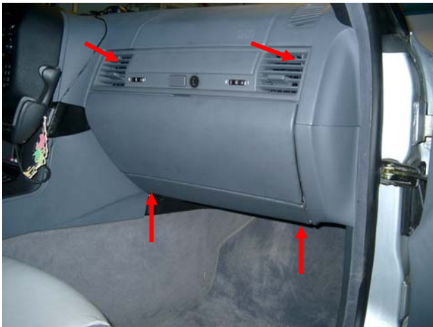
Picture 1: loosen 4 screws
