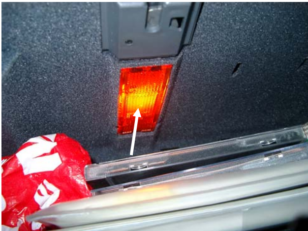
Picture 3: loosen screw behind light
