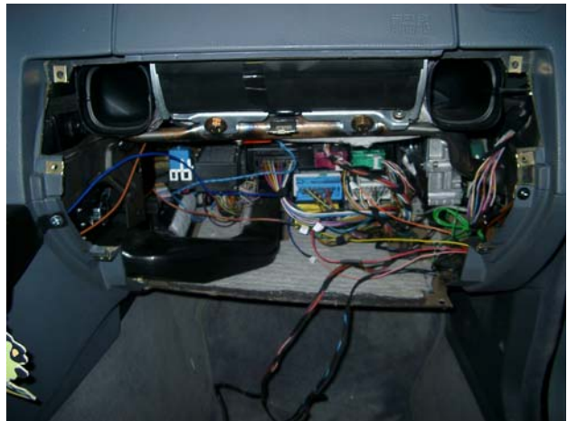
Picture 4: glove box removed
