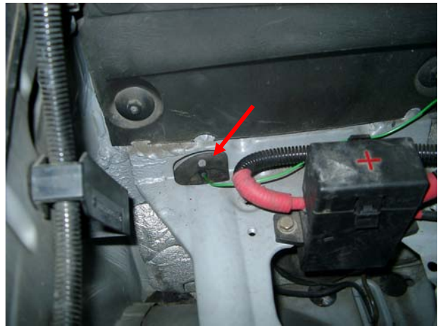
Picture 10: green wire of the relays
