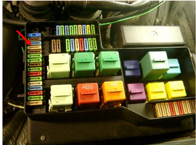
Picture 8: fuse box, fuse 43 (yellow)
