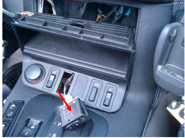
Picture 2: roof switch
