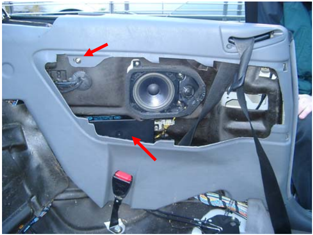
picture 2: Position BMW roof control unit
