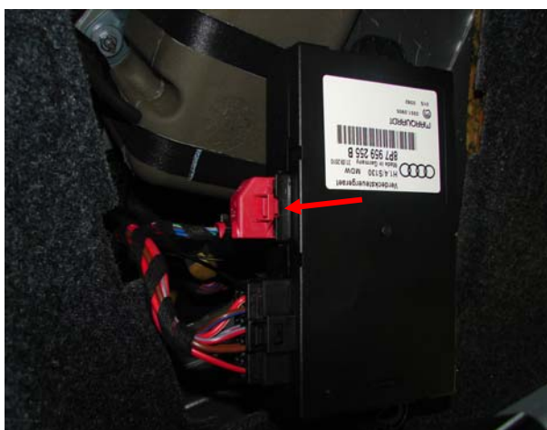
Picture 3: remove the red connector: pull down the latch (red arrow), then plug it out
