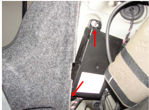
Picture 2: loosen two screws to remove the top control unit (2 nuts, see red arrows)
