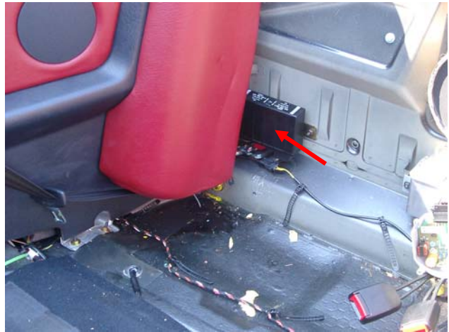
Picture 4: roof control ECU
